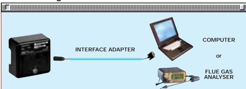
by the interface adapter and a PC with dedicated software or by a predisposed flue gas analyzer (see paragraph accessories).
