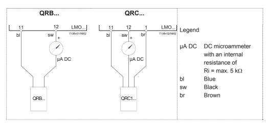
As an alternative to detector current measurement, the diagnostic tool OCI400 / ACS410 can be used. In that case, connection of the DC microammeter is not required.
