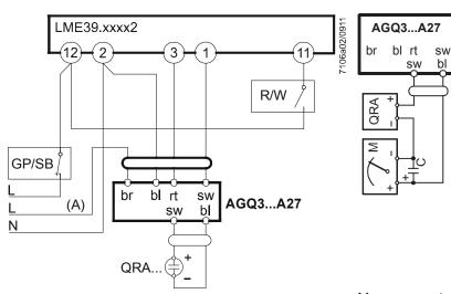
Measurement made at the flame detector QRA...
