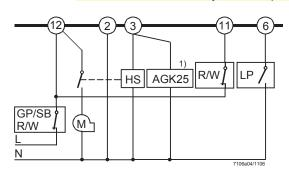
¹) AGK25 is required only if an auxiliary relay with a coil resistance of  $\geq$ 50 k $\Omega$  is used
