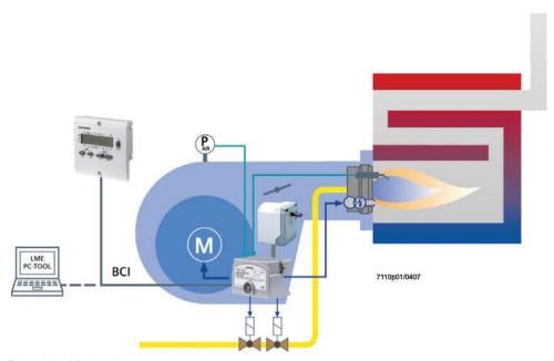
Example: Modulating gas burner
