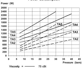
5 cSt -Rated speed = 2850 rpm Data shown are for new pumps, with no allowance for wear.
