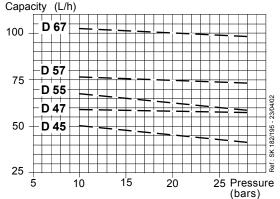
Viscosity = 75 cSt - Rated speed = 2850 rpm
