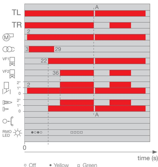
0 s The burner begins the firing cycle: the motor and transformer are supplied; the hydraulic ram opens in the pre-purge position.
